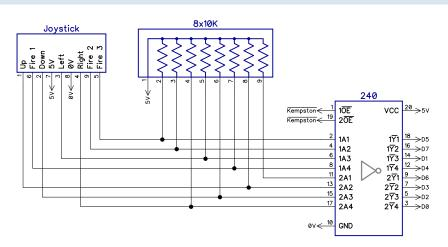
A simple 8 bit IO port is formed using the 74HC240. This is enabled by the decoded IO read from above. The 240 is an inverting buffer. The signals on it's inputs are pulled high by the resistor array and connected to the 9 way D joystick port.
