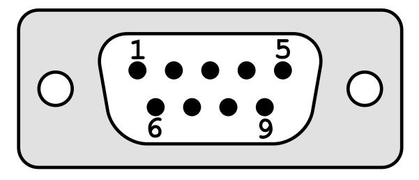
The joystick connector is the standard 9 way D pinout used on Atari and Commodore systems, and other Kempston interfaces etc. (note this is not the same as the Atari 5200, Spectrum +2 or Sega Genesis).
