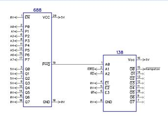
The standard address for a Kempston compatible joystick is 31 decimal, 0x1F hex.
